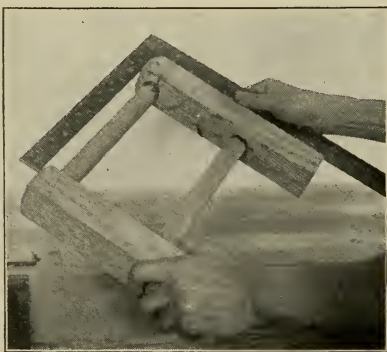
Fig. 222—Testing with Framing Square
